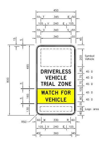
TES19715 shall be used to warn pedestrians of the Driverless Vehicle Trial Zone.
